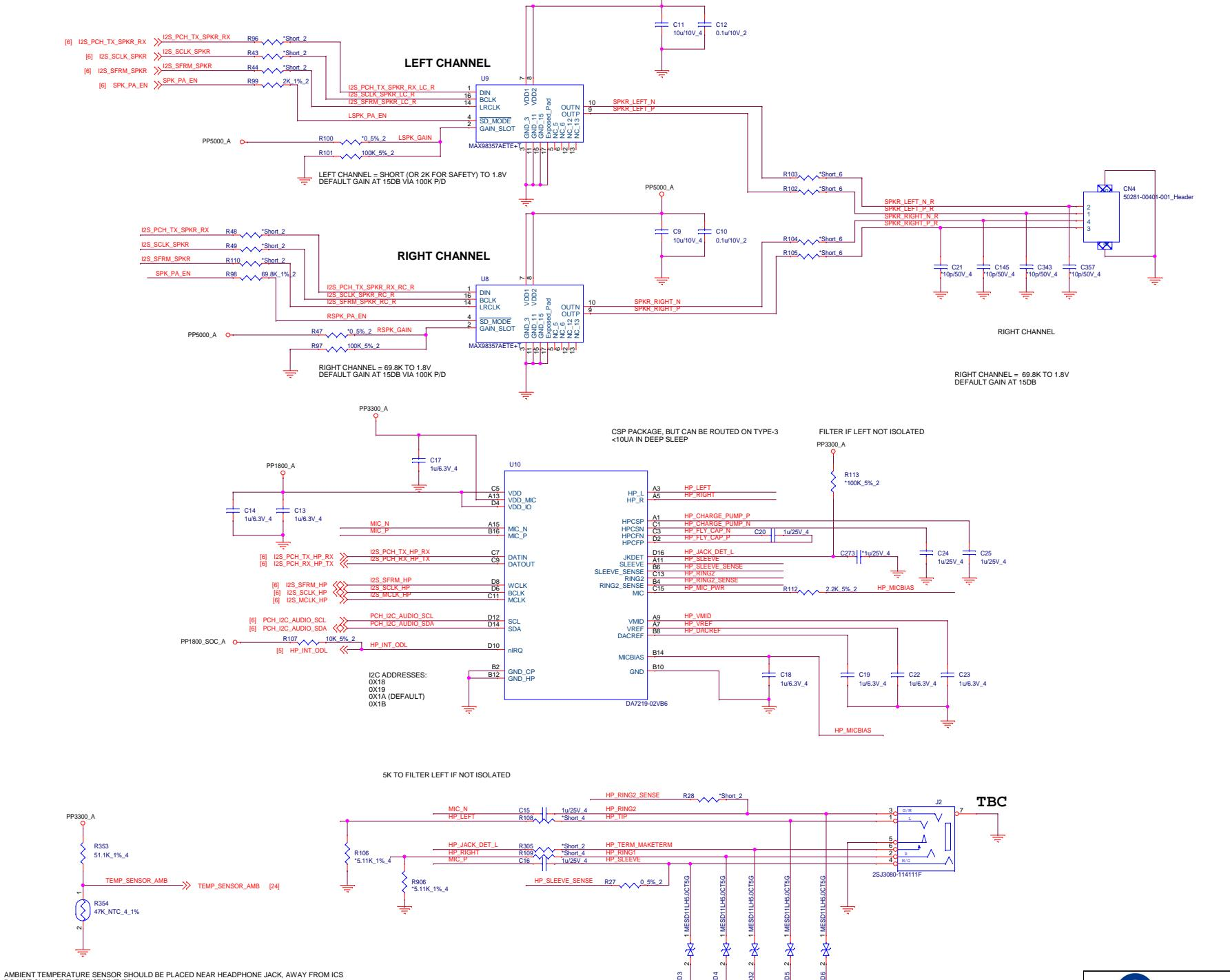
AMBIENT TEMPERATURE SENSOR SHOULD BE PLACED NEAR HEADPHONE JACK, AWAY FROM IC'S
